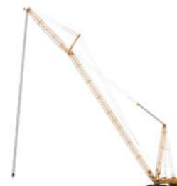
LATTICE BOOM CRAWLER
